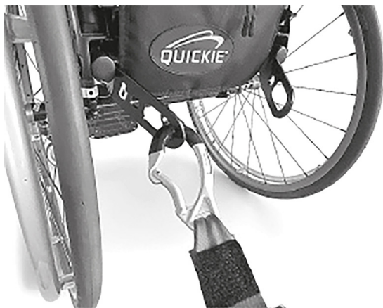
Position of the rear wheelchair tie down restraint and the tie down label.
