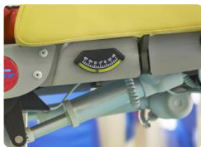
Inbuilt Inclinometers for easy re-set
