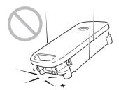
While charging, do not block the intake and exhaust vents of the charger. (When using the nickel metal hydride battery charger [JWC-2])
