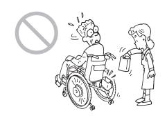
While the wheelchair is being operated or after operation, do not touch the back of the drive units. During or after operation, the back of the drive units may be hot. In addition, if the wheelchair is near a source of heat, the drive units may become hot.
