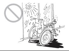
Do not wash by directly hosing it down with water. Also, do not wash with using steam. The electronic devices can get damaged, which may lead to malfunction.
