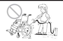
Do not clean with solvents such as gasoline or paint thinner. This may damage the painting and plastic parts.
