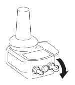
Turn the controller while the lock lever of the holder is pushed forward.
