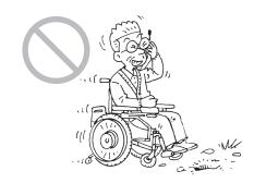
Do not operate the wheelchair near a device that produces strong radio waves. If the wheelchair is near a source of radio waves and starts to operate abnormally, immediately turn off the power, and quickly move away from that location using the assistant operations or manual operation.
