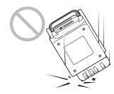
Do not use a broken or damaged battery.
