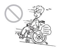
Do not operate the clutch levers while the wheelchair is in motion. There is a risk of collision or tipping over.
