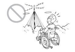
The weak electromagnetic waves emitted by the iXpress may affect other elec-tronic devices, such as automatic doors and the anti-theft systems of stores. In this case, turn off the power and operate the wheelchair using the assistant operations or manual operation.
