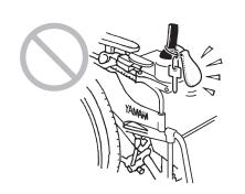
In areas with an incline, do not switch the clutch levers to the manual position. The wheelchair may start moving unexpectedly, and may collide or tip over.
