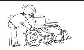
• Before using the wheelchair every day, ensure that there is air in the tires. Always keep the air pressure in the rear tires at a normal level. If the air pressure in the rear tires decreases, the parking brakes may become ineffective.
