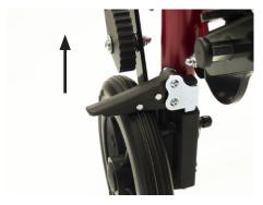
For locking, the upper clamping bracket is lowered onto the wheel pressed until the brake engages securely.
