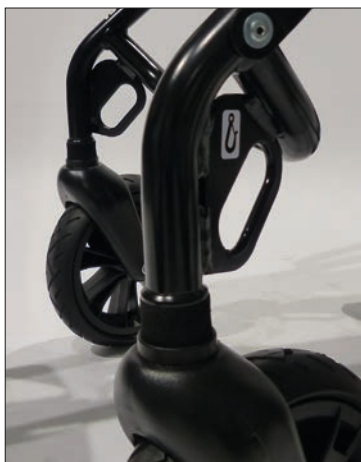
Attachment points, front according to ISO 7176-19
