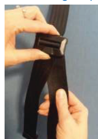
Squeeze Adjuster to release webbing
