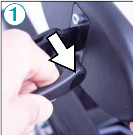
1: Pull the lever out to disengage
