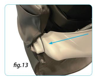
The recline angle can be read for the scale on the lower section of the back shell on the left hand side as shown in *fig.13*
