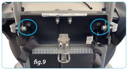
The headrest height and angle is adjusted by loosening the 4 clamp bolts highlighted above in **fig.9** once the back shell has been removed as previously described on page 8. Once loose, raise or lower the headrest in the required position, making sure the clamping blocks are at the same height on both sides. Tighten all four bolts equally until the headrest is securely locked in place.
