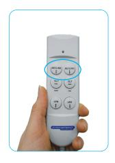
The angle of back elevation can easily be altered on the powered chair simply by pushing the buttons on the handset as shown above to alter the User's recline angle. The green light on the handset will illuminate during operation.
