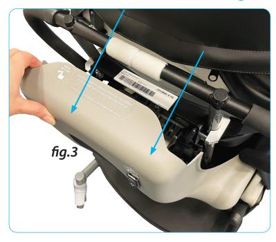
To make adjustments relating to the chair's back rest or head rest height or angle, it will be necessary to remove the chair's back hard shell casing - do this by pulling the top edge of the plastic shell away from the hook and loop fastener on the handlebar and hinge the shell backwards *fig.3* and place flat on the floor, this will expose the back rods of the chair.
