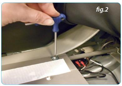
To set the seat depth, first pull the seat cushion forward as shown in **fig.1** to locate the two locking screws at the back of the seat plate **fig.2**.
