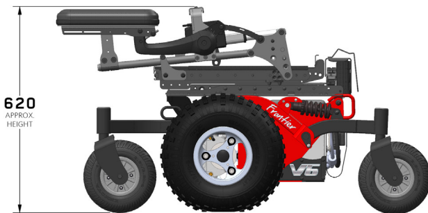
Figure 4.3c Frontier V6 and V4 Fold Forward height
