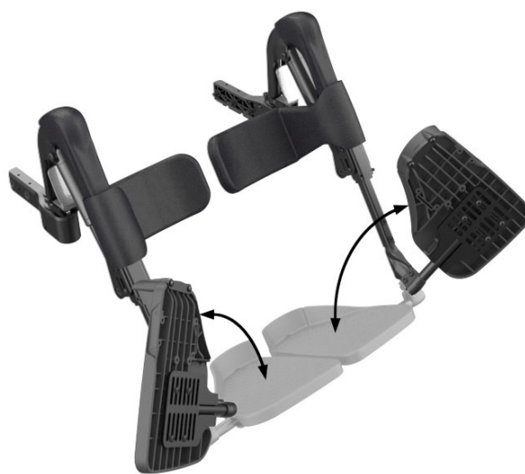
Figure 4.2c Swingaway Legrest showing removal action
