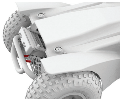
Figure 4.6b Extreme X8 brake levers released
