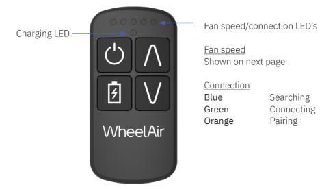
The Controller buttons function with mid (c. 3 seconds) and short (instantaneous) presses.
