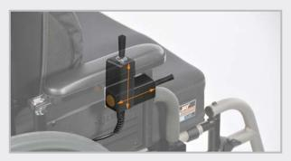
Can be mounted vertically or horizontally depending on needs. Charging port is conveniently located on the toggle switch for easy access.
