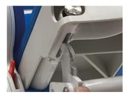
• Make sure that the openings are hooked behind the locking shafts of the seat frame.
