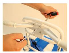
• Secure the screw connection with the supplied washers and the self-locking nuts.
