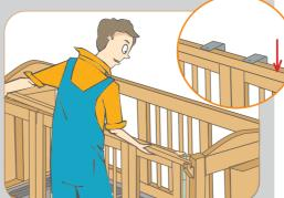
For mounting the locking bar, please put the console (17) in the drilled hole of the corner post on the head and foot side, adjust them and then secure this connection with screws.
