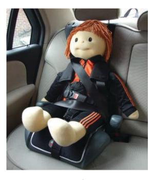
Illustrating one of our harnesses fitted in conjunction with the existing vehicle safety belt.
