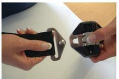
The buckle operates in reverse to the standard vehicle buckles as it is opened by raising a spring loaded lever or over-catch and **will not press release**.
